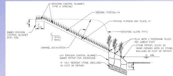
TYPICAL SECTION - REGRADE AND VEGETATE WITH BOULDER TOE
